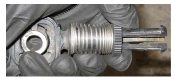
You can also grease the pins on the linkage to make the ends move smoother. Release it by lifting the center tab on the clip. I suggest doing it while it's secured to the cable so that it stays indexed to the cable end.
