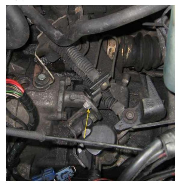
The plastic shifter linkage has also been known to break due to age and wear. To replace it, remove the adjustment nut and slip the cable off the end by lifting the retainer up. If you remove it, grease the pivots. You can also use a metal replacement that shortens the side-side throw (does not adjust the foreaft throw) with a gruvenparts assembly
