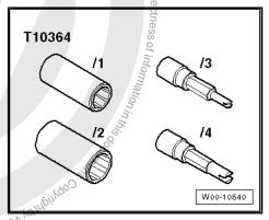
Soding lesistements to survivation of the survivati Torque wrench -V.A.G 1783- (2...10 Nm) for adapter set for service connections -T10364-
