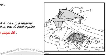
Release air quality sensor -G238- and turn to right out of retainer.
