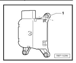
Position new left temperature flap control motor -V158marked with an "X" with shortened oval-head screw -2- and cut off bracket -1- on bracket -3- on blower box.
