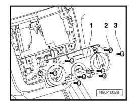
Specified torque for bolts -2- and -3-  $(1.5 \pm 0.2 \text{ Nm})$ .
