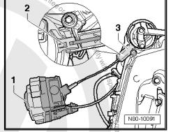
Press in locking lug-arrow- of flexible shaft and pull out flexible shaft.
