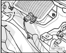
Unscrew collar nuts -arrows- (2.5 ± 0.4 Nm) and remove air intake grille upwards.
