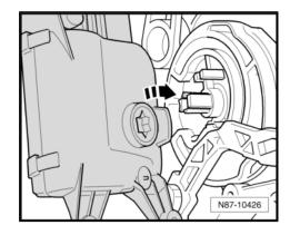
Removing and installing setting unit for fresh air and air recirculation flap and air. Volkswagen AG does not guarantee or accept you flap 3.22
