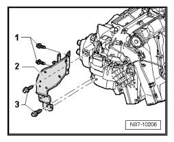
Press bracket -1- in direction of brake pedal -arrow- and secure it on brake pedal with a cable tie.
