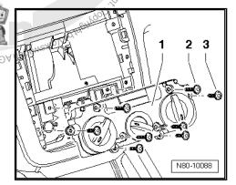
Specified torque for bolts -2- and -3-:  $1.5 \pm 0.2$  Nm.
