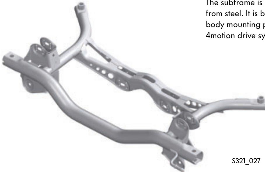
The subframe is a welded construction made from steel. It is bolted directly to the body. The body mounting points on front wheel drive and 4motion drive systems are identical.
