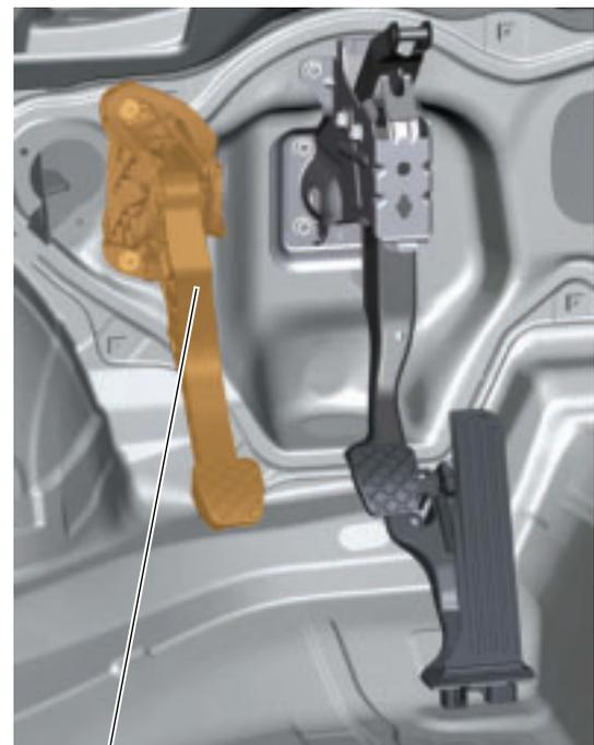
Clutch pedal with clutch position sender
