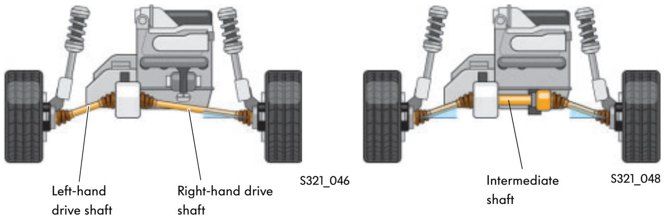
Installed in the Golf is the track proven drive shaft concept with short and long drive shafts. The shorter shaft on the left-hand side is solid. The longer shaft on the right, however, is a hollow tubular construction.
