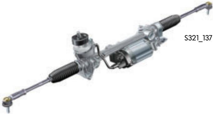
The Golf is fitted as standard with an electro-mechanical power steering system. This steering system consists of steering box and an electric motor with control unit. The system is installed on the subframe. The steering assistance from the electric motor, which is flanged in parallel to the toothed rack, is transmitted via a second pinion (drive pinion) to the toothed rack.
