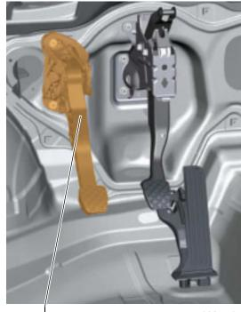
Clutch pedal with clutch position sender
