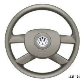
The steering wheel features a weight-optimised framework cast from magnesium. The design can be seen in the cross sectional diagram of the multi-function steering wheel.
