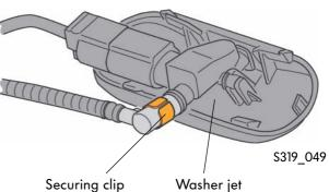
To release the connecting pieces, the securing clip must be pressed outwards by hand so that the hose can be removed.
