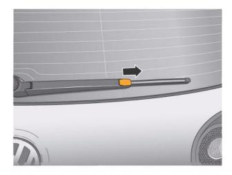
After the wiper blade has been released, the wiper arm must be lifted away from the rear window to allow the wiper blade to be removed from the mounting.
