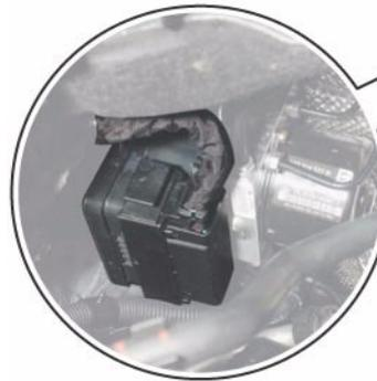
ABS with EDL control unit J104, on right of bulkhead in engine compartment
