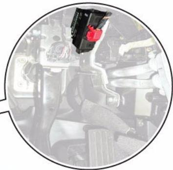
Data bus diagnostic interface J533, beneath dash panel, above accelerator pedal
