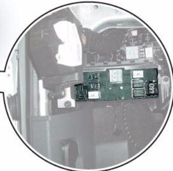
Relay carrier of onboard power supply control unit on left under dash panel
