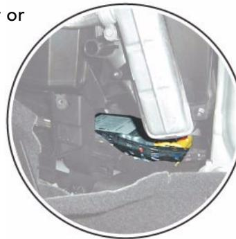
Airbag control unit J234, beneath centre console, on front of tunnel
