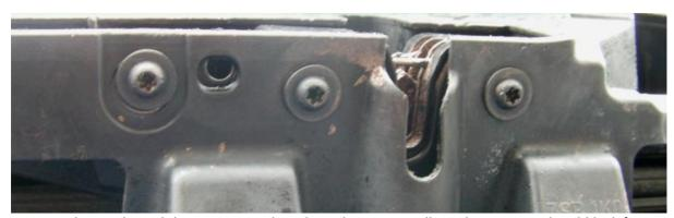
Once you have released the tension on the release lever, you will need to remove the old lock from the car
