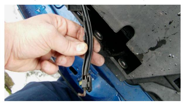
This is the plastic inside the guide, this must be fitted to the car otherwise it loses all tension in the bonnet release cable. It's used to hold the cable the correct distance and so it doesn't come loose from the car when fitting it
