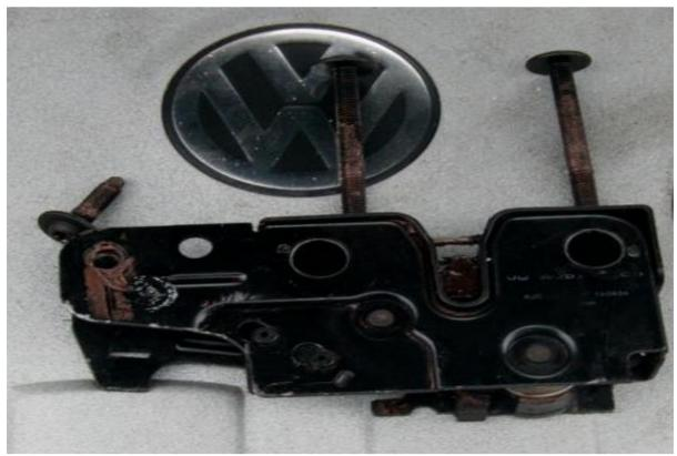
This is the layout of the T27 screws holding the lock in place on the car. There are two long ones holding the main part of the unit itself and a short one that holds the catch bar in place on the car. Make sure to fit these in the correct orientation when refitting your lock. This is a comparison to the lock placement in the above picture for future reference should it be required.
