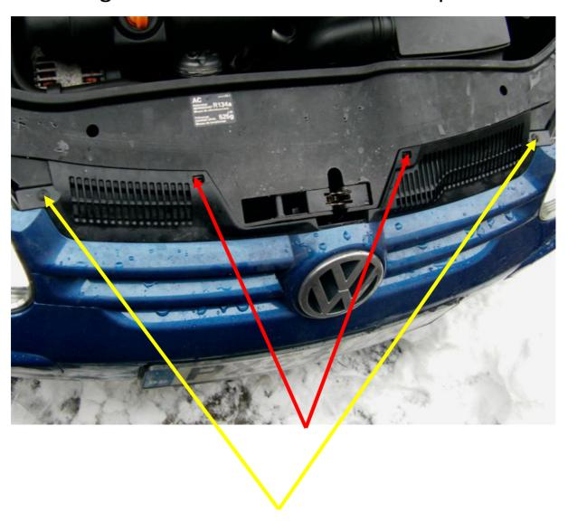
Loosen the two T20 screws here and remove them from the car {yellow}, these are the screws just next to the headlights in this picture and then once they are removed from the car squeeze in the two plastic clips {red} can do one at a time and then remove the grill from the car.
