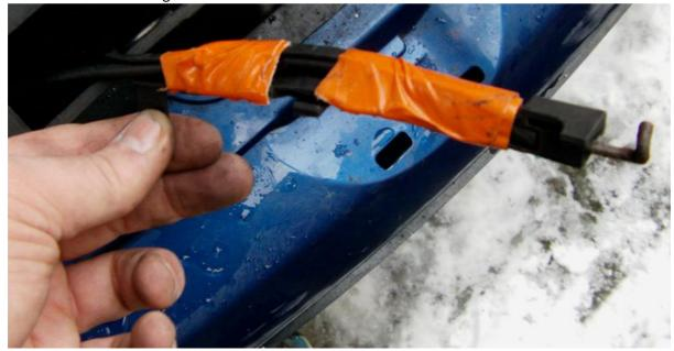
A common problem that I had when I was fitting the tensioner cable to the plastic guide was that it was slipping out and losing grip of the actual guide. This resulted in the cable losing tension and the lock not operating properly. I thought this may have been more due to not refitting the lock correctly but I didn't want to take any chances. So I bodged the lock with some gaffer tape too. This was to reduce the chances of it coming off when I was trying to refit the lock back into the housing
