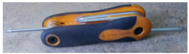
The only two tools you will essentially need for the car. A T20 and T27 torx bit. Optional tools can be some insulation tape to hold the plastic guide in place as I found mine kept coming loose every now and then when refitting it to the car aswell as some zip ties and a flat-head screwdriver if you don't have good pinching grip with your fingers.
