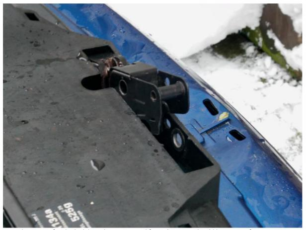
Once the screws for the lock have been removed from the car, it should be a case of extracting it. There is no real tension to it, you should be be able to remove it just by pulling on the normal piece of metal where the bonnet lock catches onto when you shut it after this it's just a case of extracting
