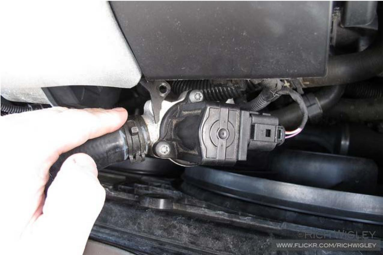
Now is a good time to remove the electrical connector from the DV, just push the tab down and pull it off.
