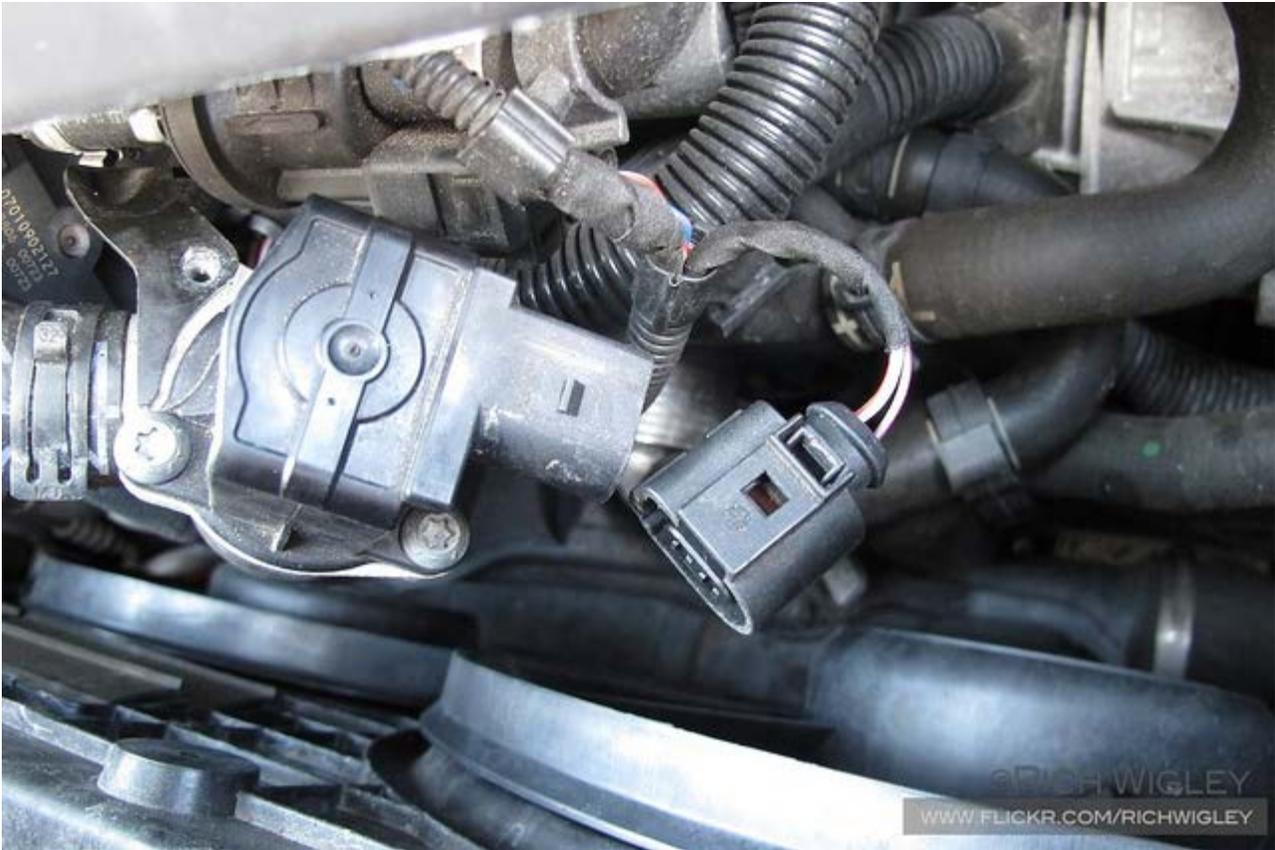
Starting with the bolt on the right (as shown below) remove the three bolts one by one in a clockwise direction.
