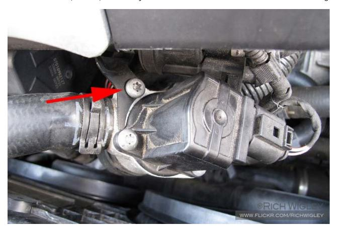
Removal of the bolt allows you to move the DV toward the front of the engine bay so you can access the other 3 torx 30 bolts.
