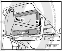
This is a view of the monitor with the plastic pin -arrow- disengaged.
