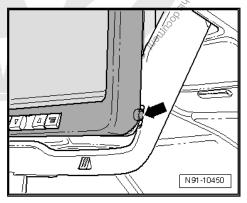
Tilt monitor so that the guide pins -arrows- can be guided out of the guide rails.
