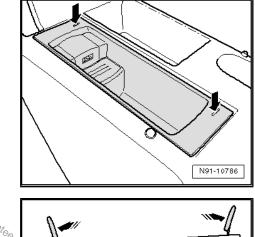
Push the release tools apart in direction of -arrow- to flawlessly release the locking mechanism. With the release tools still pressed, pull the complete insert out of the centre armrest.
