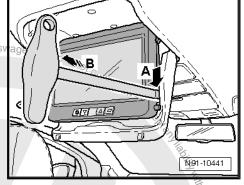
Carefully pull monitor using front-end hook -VAS 3370- in direction of -arrow A- until the plastic pin disengages.
