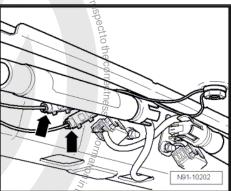
Release connectors -arrows-, disconnect them and remove roof aerial.
