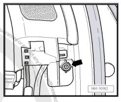
If the plastic clip -arrow- is still on trim panel after removing, take it off and fit it in the appropriate position in the door.
