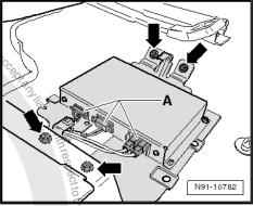
Remove bolts -arrows-, counterhold nuts under retainer, otherwise these will also turn. viviate of commercial purposes.
