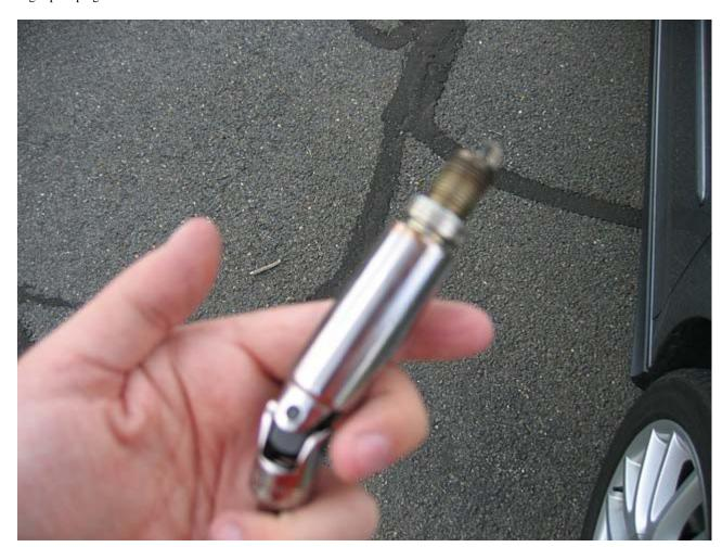
To install the new plug, take the old one out of the socket, push the new one in, then reverse the steps.
