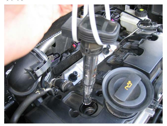
With the coil pack out, hook up your plug socket and extension and feed the end down into the hole.
