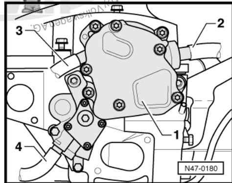
**Exhauster pump for 4-cylinder diesel engine (4-valve):**
