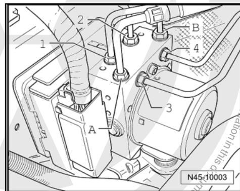
**6.2.3 Unbolting control unit from hydraulic unit**
