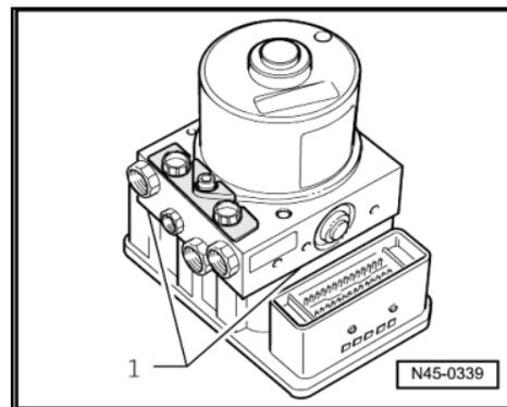
When pulling off the control unit, ensure that the hydraulic unit contact pins are not canted against the control unit solenoids.
