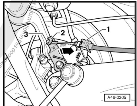
Handbrake cable -2- must be installed without tension between brake caliper bracket and fastening clip.
