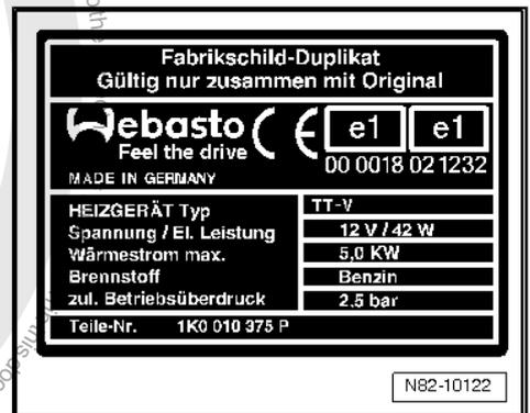
**Manufacturer's plate (duplicate) on lock carrier for Thermo Top V, diesel (preheater without auxiliary heating function)**
