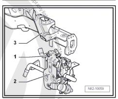
Remove securing nut -1- (15 ± 1.5 Nm) from auxiliary heater -2- on right longitudinal member -3-.
