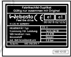
Manufacturer's plate (duplicate) on lock carrier for Thermo Top V, . DA negswexlo V to Ing. diesel (preheater without auxiliary heating function) Protected by co
