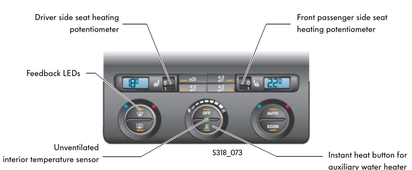
In the case of the Climatic operating unit, the button "AC" has been renamed "ECON".
