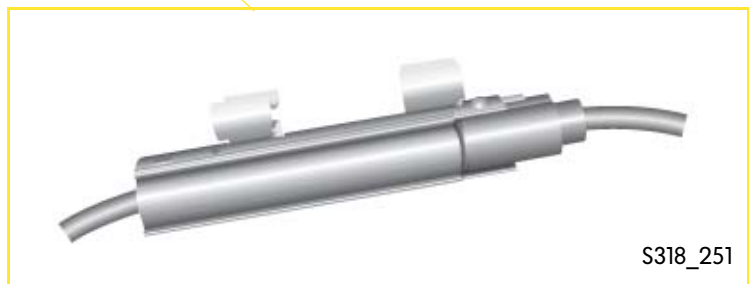
Disconnection point closed
