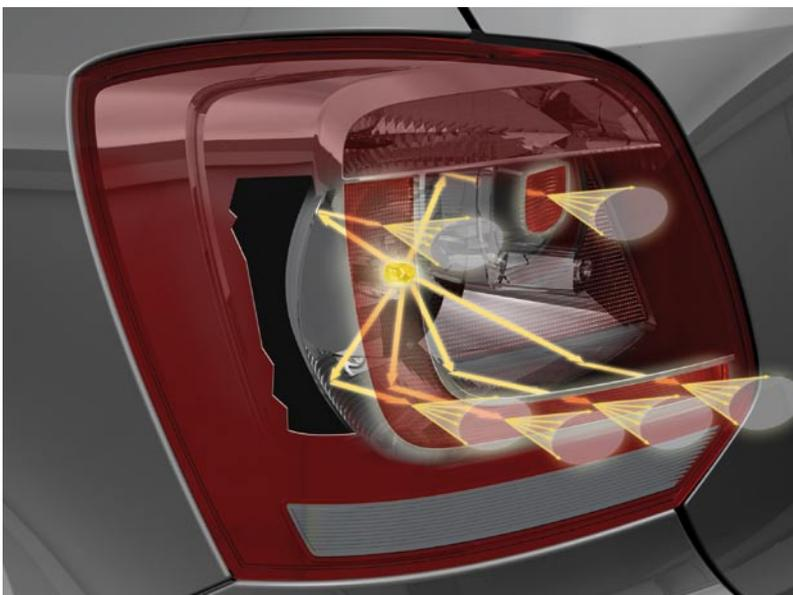
Figure 4: Sectional view of the light with beam path (optical concept)
