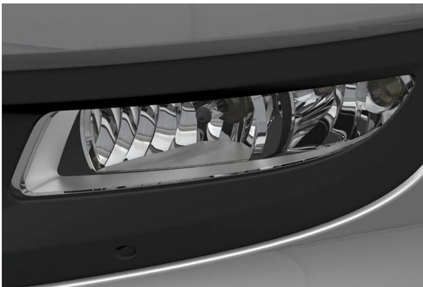
**Figure 1:** Light module in bumper with fog lamp, cornering light and daytime driving light function
