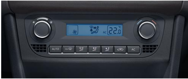
Figure 10: Air conditioning control
