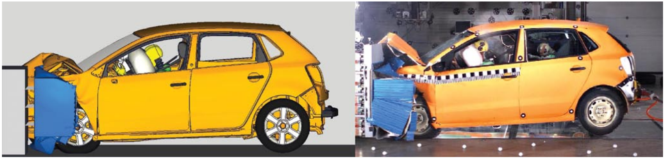
Figure 4: EuroNCAP front-on collision; comparison between simulation and test
