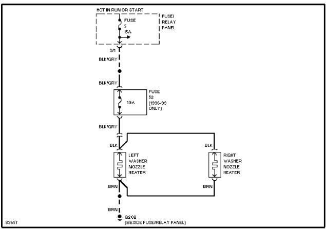
Heated Windshield Washer Circuit
