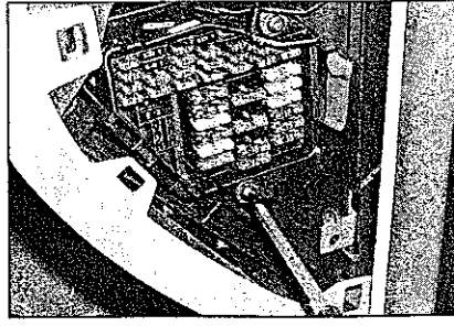
30.9 Remove the two fusebox securing screws
